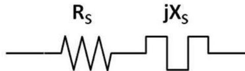
FIGURE 2. A simple equivalent circuit for inductors with ferrite cores. jX_S represents the lossless inductive reactance and R_S represents resistive loss. Both jX_S and R_S change with frequency.
